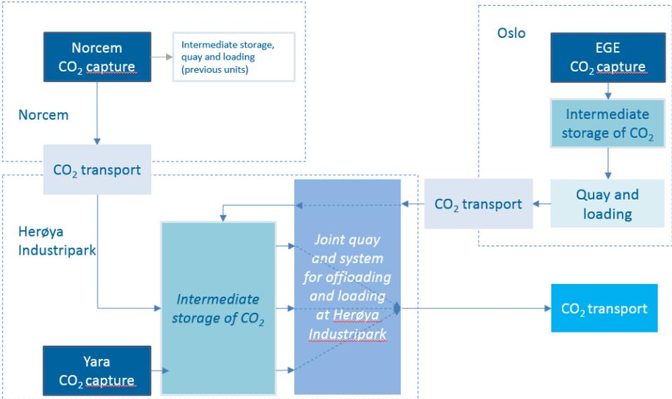
Figure 5.6.1 Joint CO<sub>2</sub> intermediate storage site in Grenland.
