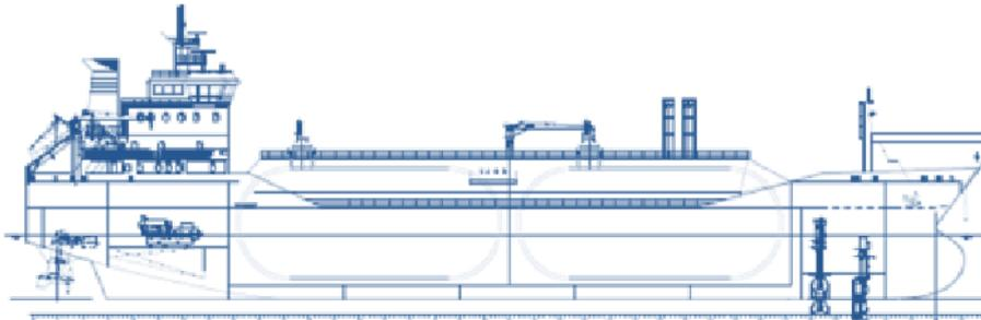
Figure 6.2.1.1 Low pressure, transport volume 6 000 m<sup>3</sup>–7 700 m<sup>3</sup>, ship length 114 m–150 m.
