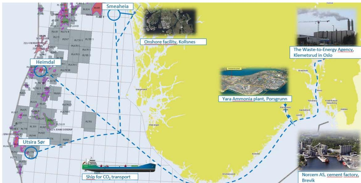
Figure 3.1 Illustration of CO<sub>2</sub> chains assessed in the feasibility study.
