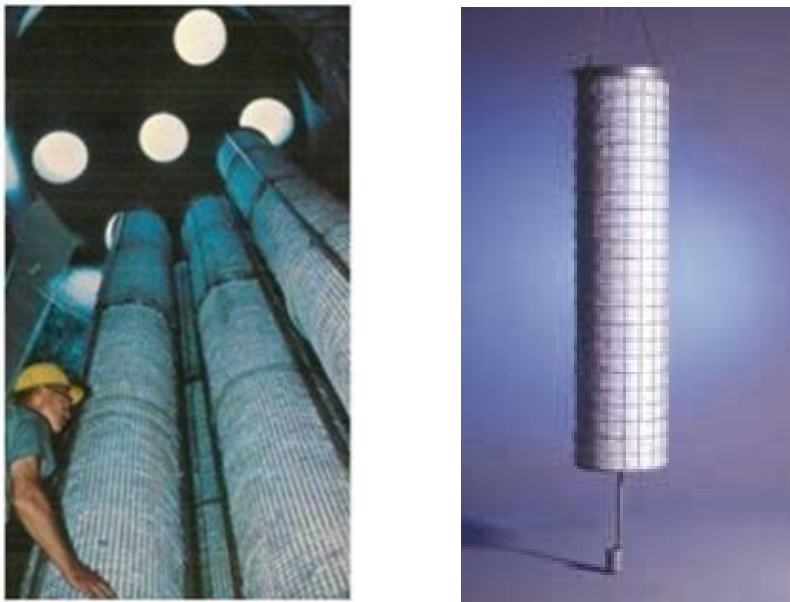
Figure 3.17 Brownian diffusion candles (Brink packed glass fibre filters)
