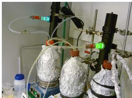
Figure D-2: Laboratory setup developed to study proof of principle destruction of N-DELA
